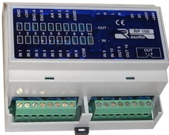
Compact mini-PLC module for small automatic machines control. It has good processing speed, 10 digital inputs, 10 digital outputs, 1 encoder position control, 2 +/- 10Vdc analog outputs, 2 RS-485/Can-BUS serial ports, lithium battery date clock, operation diagnostics using front LED rows, connection sockets for operator panels.
